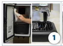
Using a clean, damp cloth, clean the external cabinet and splash areas including door-gasket.
