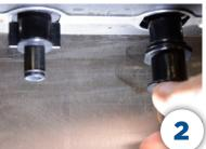
Remove dispense nozzles by rotating each 90° and pulling down. Wings on the nozzle must be facing the front of the unit to remove.
