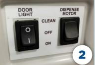
Set dispense motor switch on back of the door to "Clean Mode"
