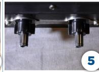
Reinstall each nozzle by inserting with wings facing the front of the unit, push upward, then rotate 90°.
