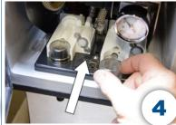
Reinstall mixing chambers by pushing straight forward.
