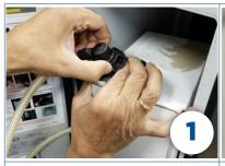
Disconnect product output connector from BIB (Bag in Box product) by turning the black threaded connector counterclockwise and lifting on the outside of the black connector.
