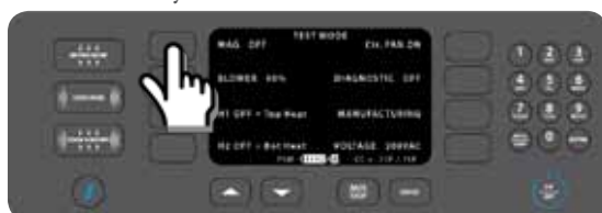
Figure 17: Test Mode: Magnetron Test
