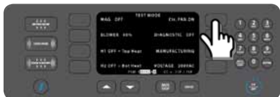
Figure 23: Test Mode: EC Fan Test
