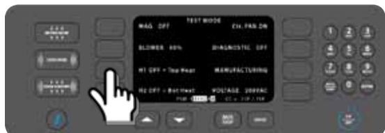
Figure 21: Test Mode: Top Heater Test
