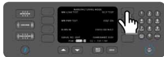
Figure 31: Select “Self Test”
