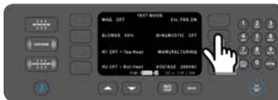
Figure 24: Test Mode: Diagnostic Mode On/Off
