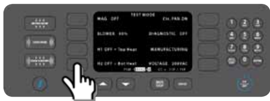
Figure 22: Test Mode: Bottom Heater Test
