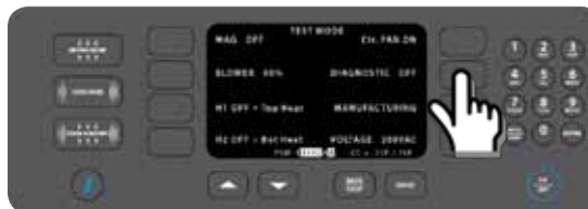
Figure 25: Test Mode: Select “Manufacturing Mode”
