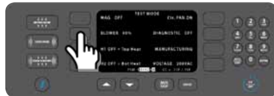
Figure 19: Test Mode: Blower Test
